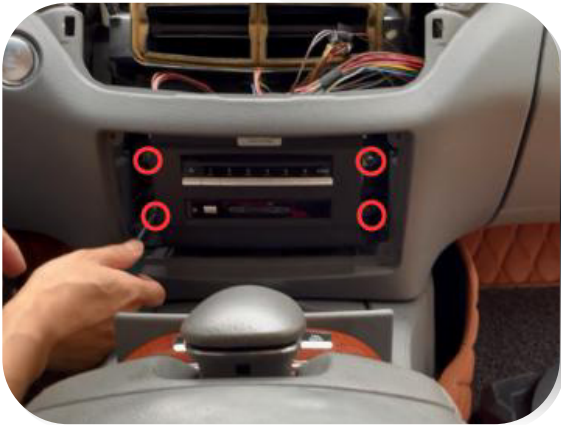
26.Loosen the screws of the OEM player
