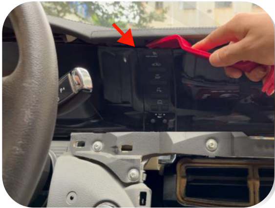
14. Pry out the control panel
