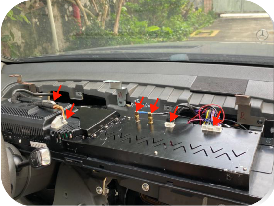
39.Plug in the OEM instrument cluster and android screen
